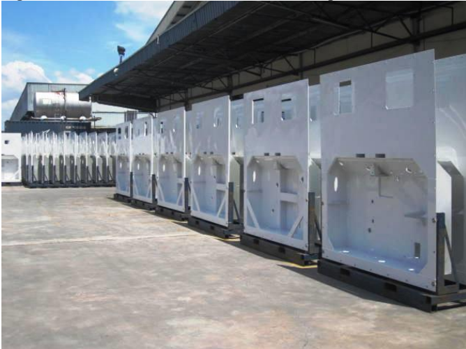
Figure 3. Aluminium frames for container refrigeration units
