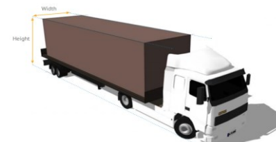
Figure 3: Transportation of PPVC by trucks
