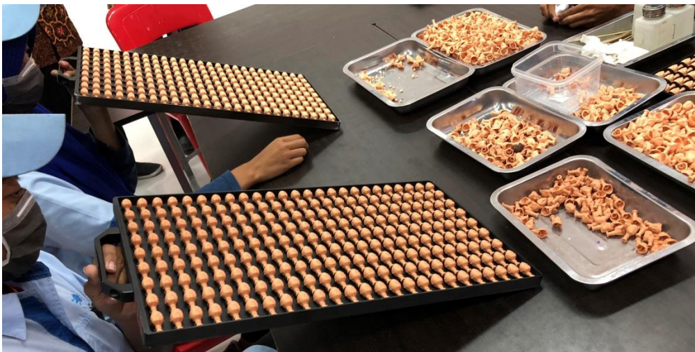
Figure 5: Workers placing doll head (without eyes) on to the holding plate for printing
