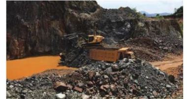
Figure 23: Removal of blasted materials
