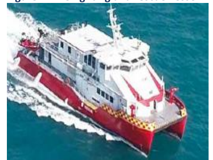
Figure 4: Fire fighting and rescue vessel
