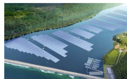
Figure 27: Artist impression of the upcoming 60MWp floating solar system on Tengeh Reservoir occupying an area of about 45 football fields
